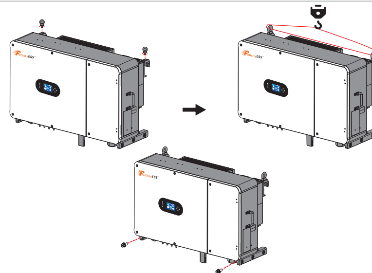
Figure 3.4-2 Installing an Inverter
